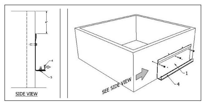
**6.** Using approved sealant – seal the sheet metal joints on the exhaust fan.
